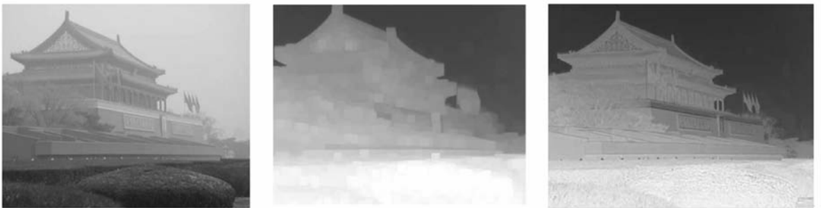
(a) 原始雾化图像 (b) Kaiming He 的透过率 t 估测图 (c) 本文的透过率 t 估测图 (a) Original hazy image (b) Estimated transmission map for (a) by Kaiming He (c) Estimated transmission map of for (a) by proposed method
